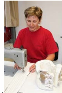
Handcraft: This picture shows how the self-produced heating cables with the corresponding isolations are sewed into a backing fabric of mats and jackets.
